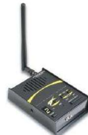
Mobile and Base station radios are usually more powerful than hand-held radios and may have as much as 100 watts of power.
