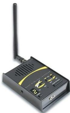
These call boxes use either UHF or VHF frequencies to communicate over long range. Most of these wireless frequencies require an FCC license, but the VHF version has the unlicensed MUR frequencies as well. These call boxes can be programmed to be compatible with virtually any brand of VHF or UHF business band radio.
